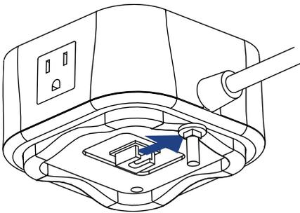
4. Thread the mounting nut onto the mounting bolt and tighten until the power station is snugly in place.
