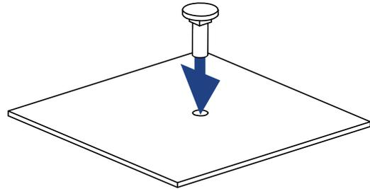
3. The power station has an area to grip the mounting bolt. Align with the screw and slide the power station onto the bolt.
