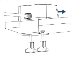
2. Twist hand knobs until power station is secured
