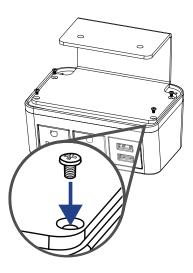
3. Thread hand knobs into mounting bracket
